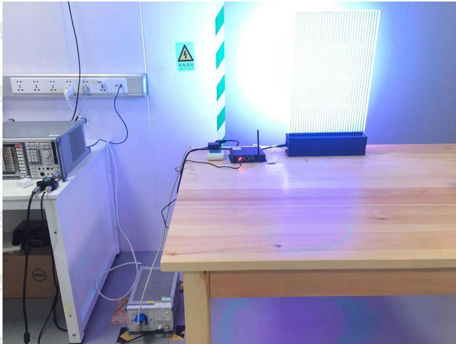
Photo 5 Power Line Conducted Emission Test
