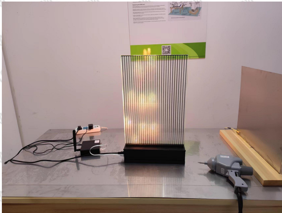
Photo 6 Electrostatic Discharge Test
